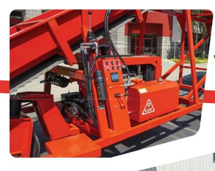
A powered drive wheel with a large flotation tire and smooth steering helps position the 3690 where you need it
