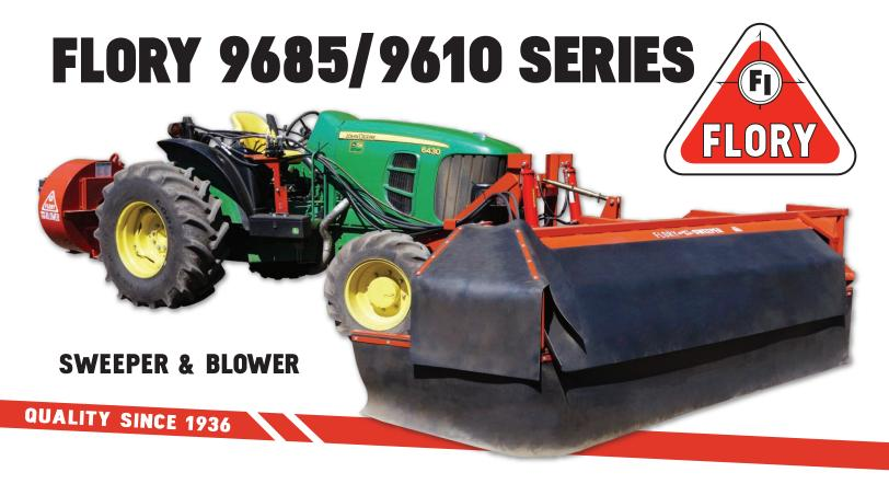
**THE FLORY 9685/9610 SWEEPER SERIES & 2500 BLOWER** is used for walnut, almond, pecan and fig orchards. It provides fast and effective sweeping and blowing in heavy trash conditions. The reel type sweeping head has proven superior in loose and sandy soils and in heavy grass. It is available with a self-contained hydraulic system, which eliminates the need for additional mountings of pumps as well as various other benefits. Flory Quality above all.
