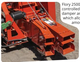
Flory 2500 Blower is controlled with a damper and cylinder which allows a variable amount of air
